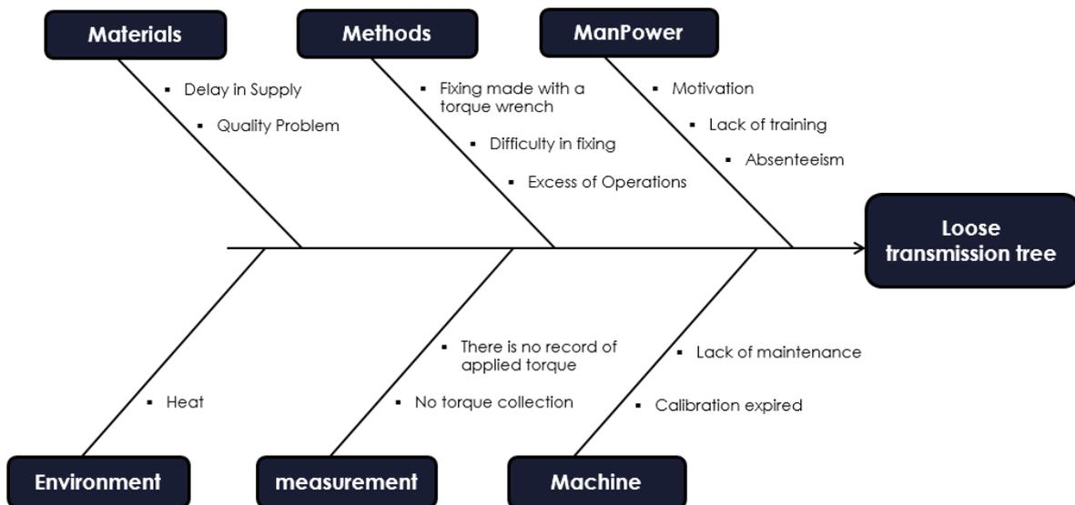
Fig. 5. Fault: Loose transmission tree.
