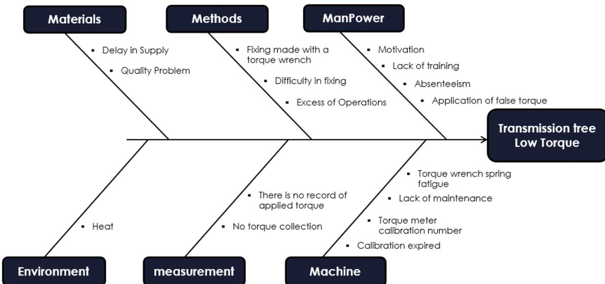
Fig. 6. Fault: Transmission shaft with low torque.
