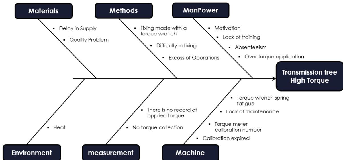
Fig. 7. Fault: Transmission shaft with high torque.
