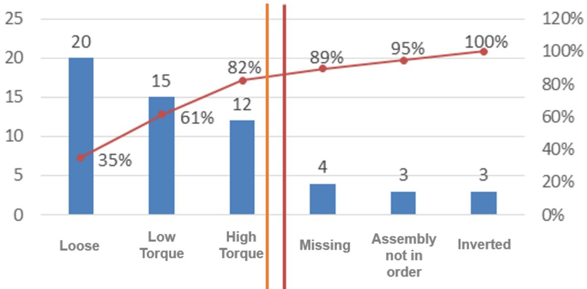
*Fig. 4. Pareto Graph of Operational Failures of Transmission Tree Subsystem.*
