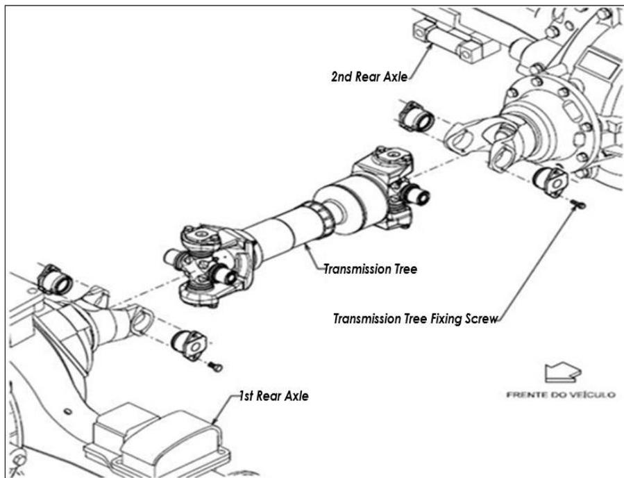
Fig. 3. Assembly of cardan between the rear axles of a 6x4 vehicle.
