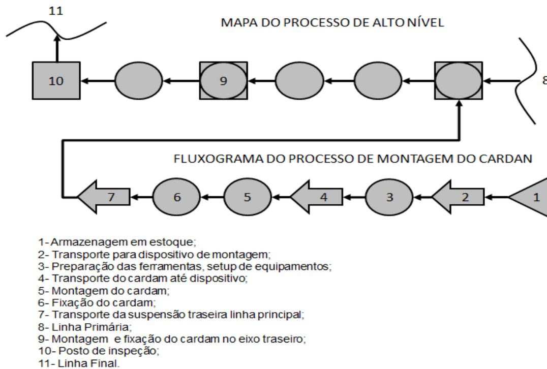
Fig. 8. Process flowchart of the cardan mounting station between the axes and the chassis line.
